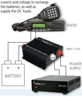
**SPECIFICATIONS** Output Amps Weight Dimensions Input Model (VAC) (VDC) (lbs) (inches) Compliance (A) SEC-1223BBM 120 13.8 23 3.4 7.0 x 9.5 x 2.4 UL. FCC SEC-1223BBM-CE 230 13.8 23 3.4 7.0 x 9.5 x 2.4 CE
