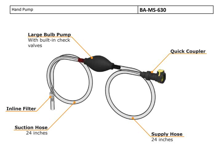
This water supply is perfect for the person who has their own golf cart, utility vehicle, or other light use application. It is commonly used with a jug filled with distilled water. The hand pump is for use with batteries that feature 24 or fewer cells and are equipped with Millennium SPW, Pro-Fill, or Qwik-Fill systems.
