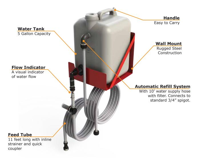
Gravity tanks may be put on a shelf or used with our rugged mounting bracket. Bottom of tank must be at a minimum of six feet above the top of the batteries being watered. Tank automatically refills itself. Compatible with deionized water.
