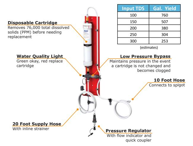
Maximizes battery life by removing ions and heavy metals that are present in tap water. The separate bed deionizer uses an ion exchange cartridge to filter the water before it enters the battery. Cartridge can be discarded when replacement is necessary. This is determined when output exceeds 50 TDS (water quality light will turn red). The low pressure bypass ensures that the deionizer will provide enough pressure and flow to operate your SPW system, even if your cartridge becomes plugged.
