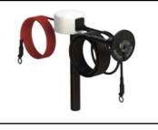
Eagle Eye Remote Standard is used on 11-33 plate batteries where the battery top is not easily viewed. The remote light mounts on the dash or the side of the battery case. It is frequently used on narrow aisle lift truck batteries that remain inside the vehicle and are not readily accessible. 1.93" / 49mm (Standard length) BA-494
